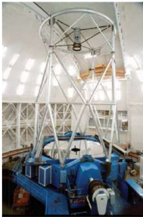
Figure 4.18 Optical telescope modal test with 100 accelerometers and multiple impact locations, showing time streamed data collection for three accelerometers and 25 samples acquired.
