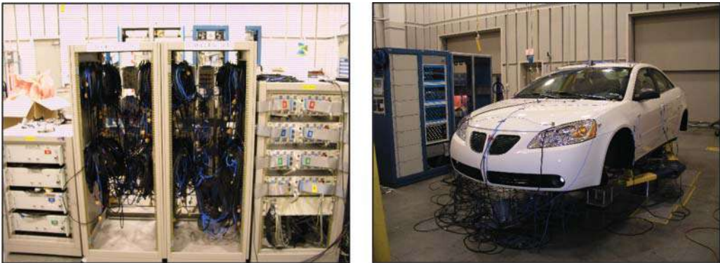
Figure K.1 Typical automotive modal test setup.
