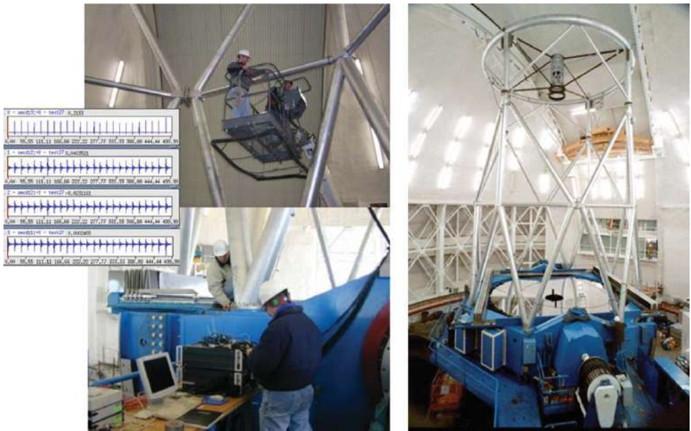
Figure 7.6 Modal and operating testing on a large optical telescope.
