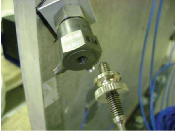
Figure 8.8 Structure shaker misalignment requiring shaker adjustment.
