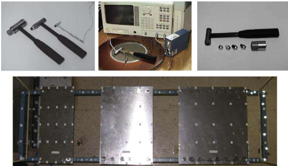
Figure 4.19 Typical impact measurement setup for blue frame structure.
