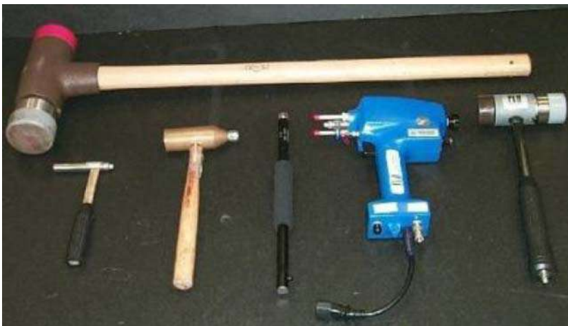
Figure 11.1 Assortment of commercially available impact hammers. Image courtesy of PCB Piezotronics, Inc.
